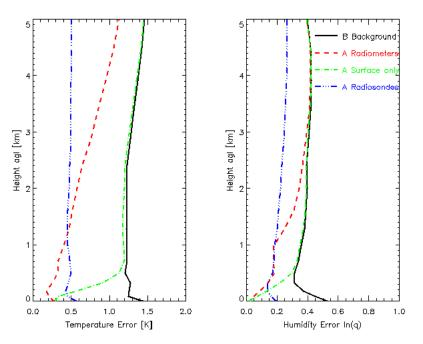
**Figure:** Uncertainties on background from mesoscale model (black) and retrieved profiles, using surface sensors only (green), MWR and surface sensors (red), and radiosonde only (blue). Left panel: temperature. Right panel: specific humidity (adapted from Hewison and Gaffard, 2006).
