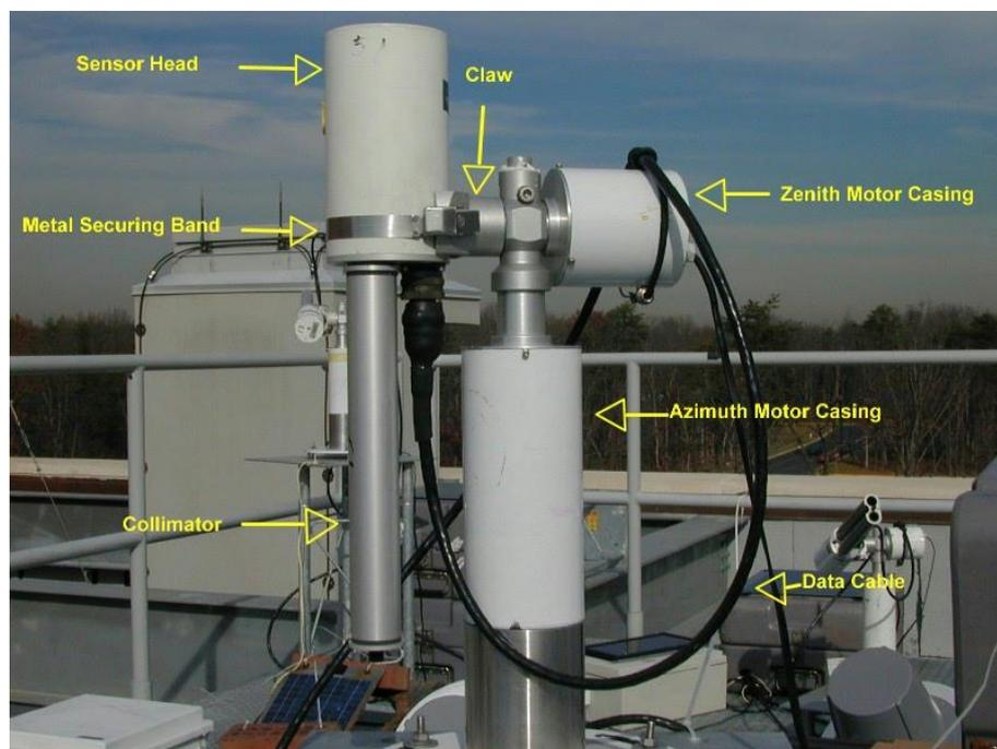
Figure 3: Picture showing a CIMEL sun photometer with sensor head and data cables attached (Source: AERONET website).
