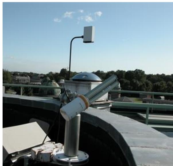
Figure 2: Both images show a CIMEL sun photometer installed on the roof at BIRA-IASB in Brussels (source: AERONET website).
