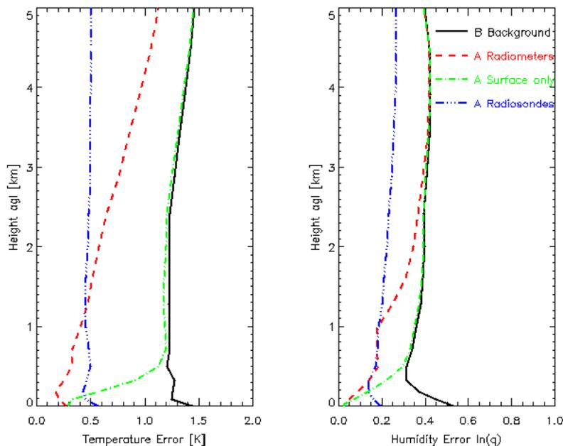
**Figure:** Uncertainties on background from mesoscale model (black) and retrieved profiles, using surface sensors only (green), MWR and surface sensors (red), and radiosonde only (blue). Left panel: temperature. Right panel: specific humidity (adapted from Hewison and Gaffard, 2006).
